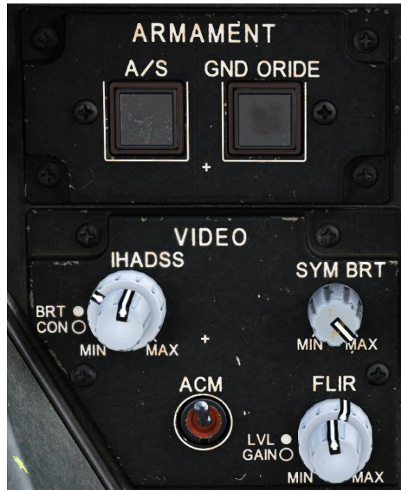
Figure 23. Armament and Video Panels
