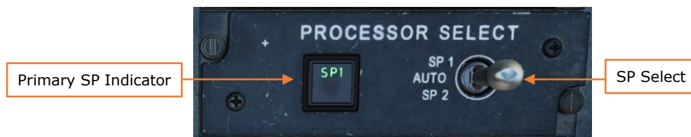
Figure 50. Processor Select Panel
