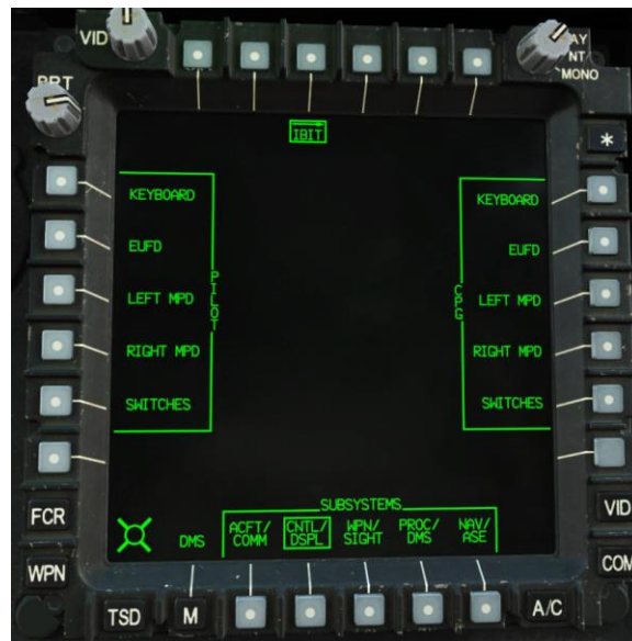
Figure 134. MPD DMS Page, IBIT Sub-Page, CNTL/DSPL Format
