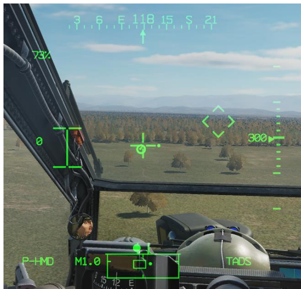
Figure 266. HMD Rocket Engagement – Pilot HMD LOS reticle on target
