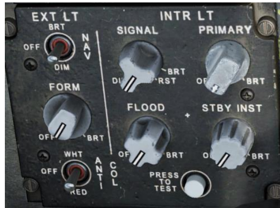
Figure 31. Exterior/Interior Lighting Panel
