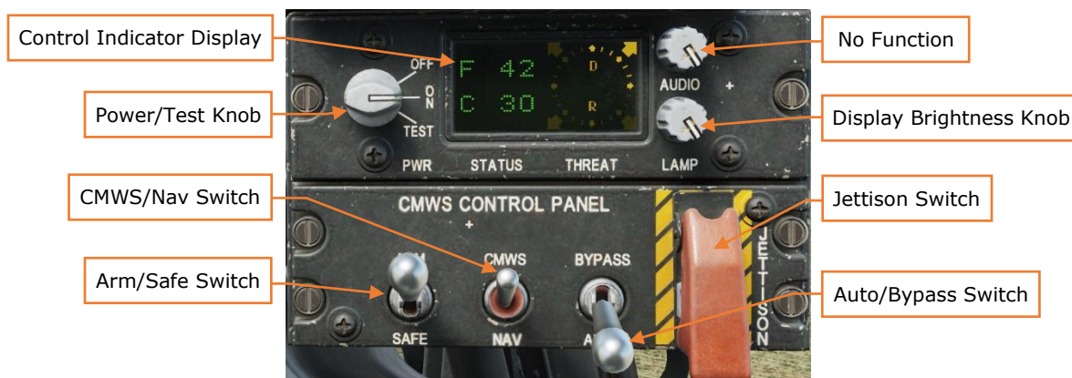
Figure 300. CMWS Control Indicator
