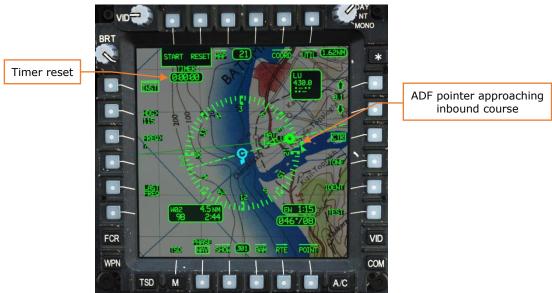
Figure 210. INST Sub-Page, Turning to the Inbound Course
