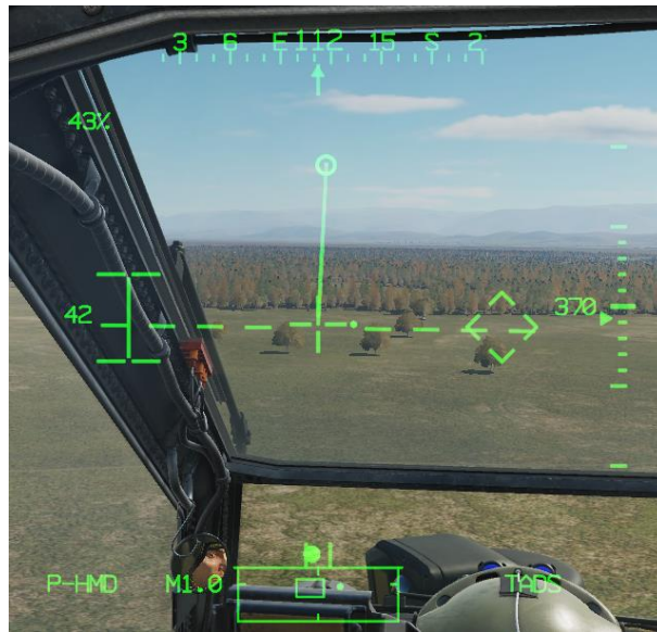
Figure 269. HMD Rocket Engagement – Pilot HMD LOS reticle on target
