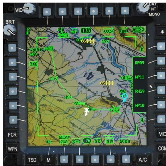
Figure 195. Additional Points added to a New Route
