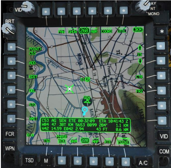
Figure 178. POINT Sub-Page, ADD Menu, Point Manually Entered
