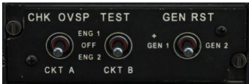
Figure 34. Check Overspeed Test/Generator Reset Panel
