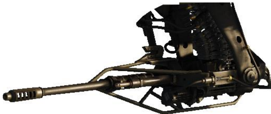
Figure 6. M230 Area Weapon System
