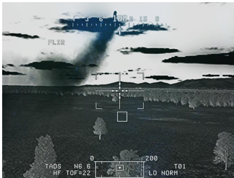
Figure 294. TADS Remote Hellfire Engagement – Time of flight displayed
