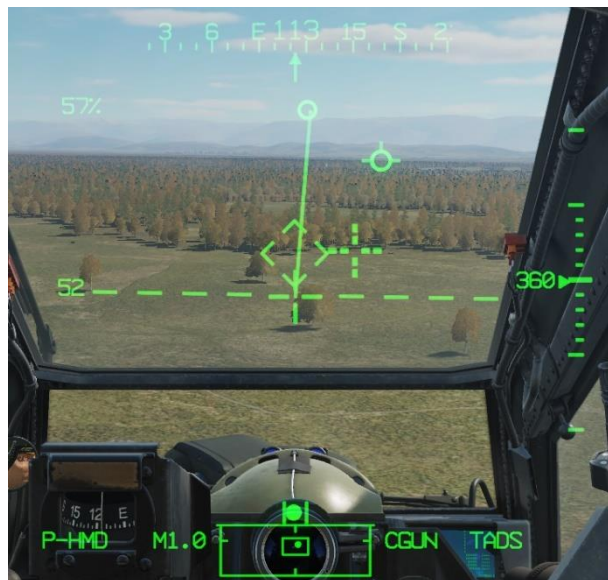
Figure 244. TADS Gun Engagement – Pilot HMD symbology
