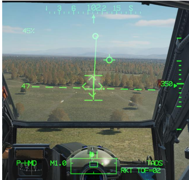
Figure 271. HMD Rocket Engagement – Rocket Steering Cursor alignment
