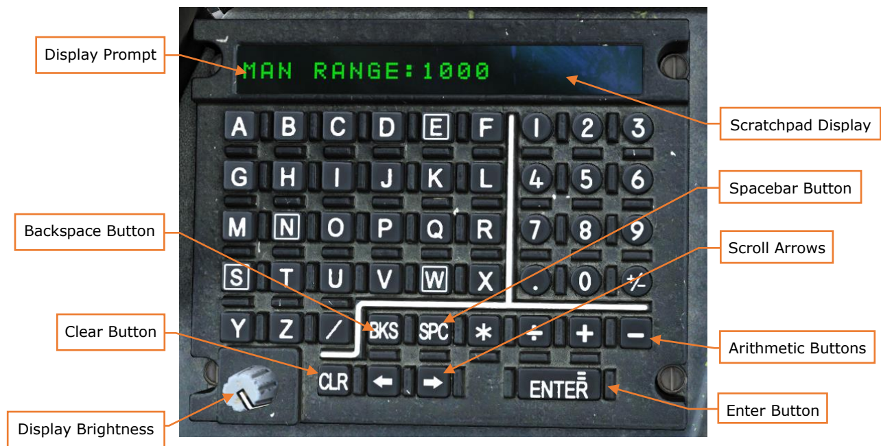
Figure 144. Keyboard Unit with Prompt
