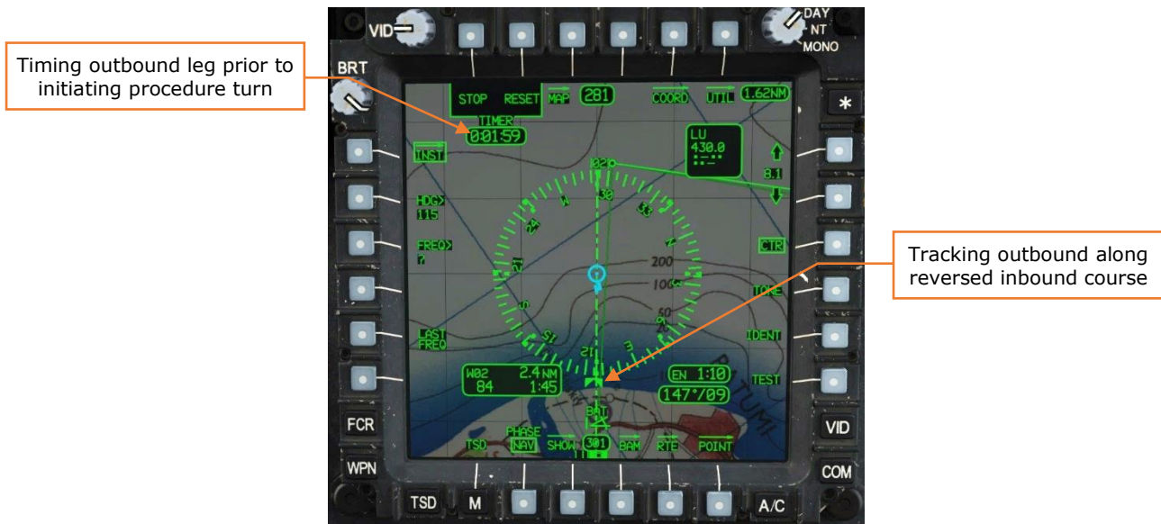
Figure 214. INST Sub-Page, Tracking Outbound from the NDB
