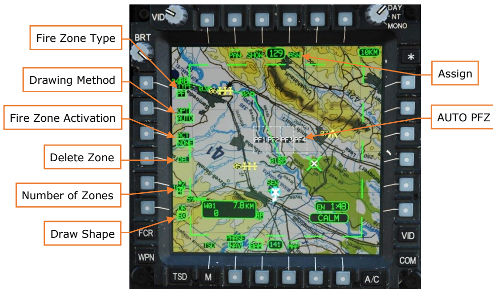
Figure 90. MPD TSD Page, BAM Sub-Page, PF Format (AUTO Option)
