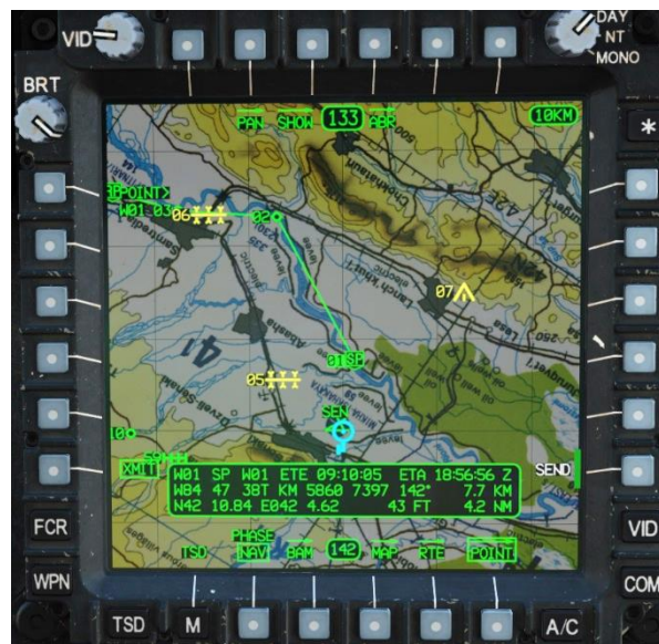
Figure 187. MPD TSD Page, POINT Sub-Page, XMIT Menu
