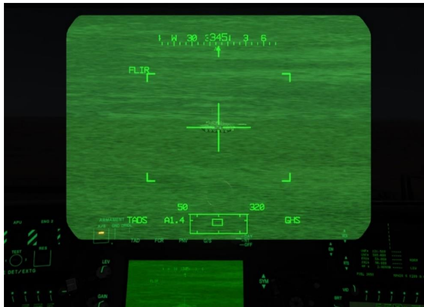
Figure 228. CPG HDU with Weapon Symbology & TADS Sensor Video
