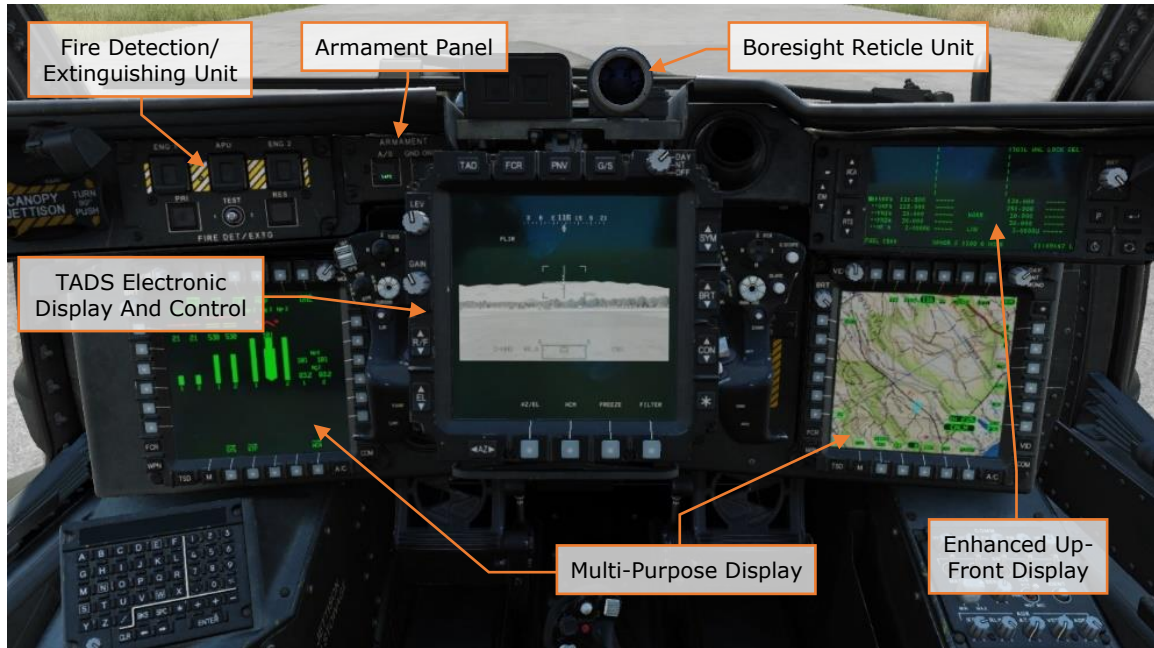
Figure 43. CPG Cockpit, Forward
