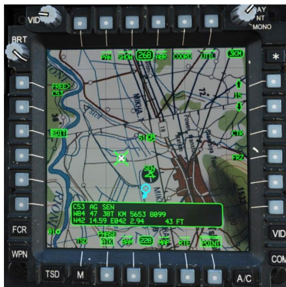
Figure 179. POINT Sub-Page, EDIT Menu, Point Selected
