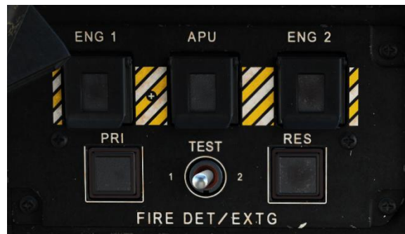
Figure 22. Fire Detection/Extinguishing Unit
