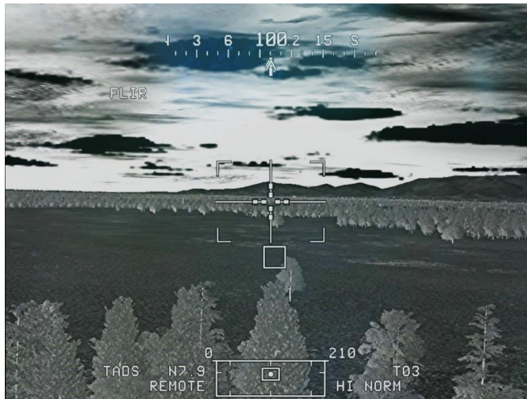
Figure 297. TADS Remote Hellfire Engagement – CPG TADS Video
