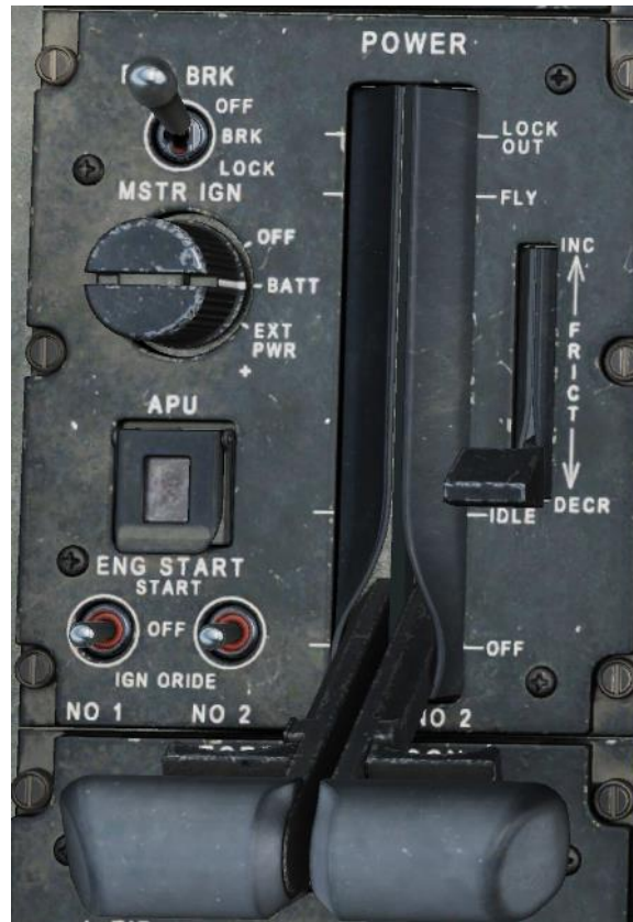
Figure 29. Power Lever Quadrant
