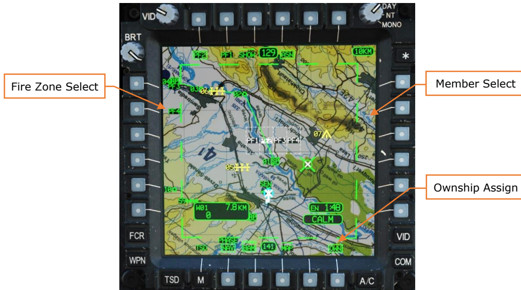
Figure 96. MPD TSD Page, BAM Sub-Page, PF Format (ASN Menu)
